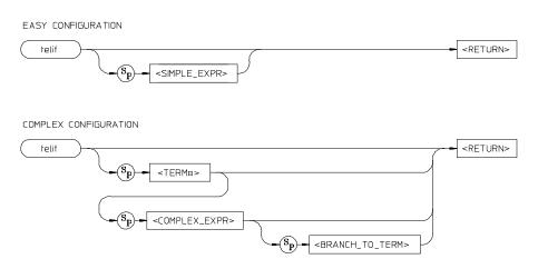
The **telif** command allows you to set the global restart qualifier (in easy configuration) for the emulation-bus analyzer sequencer. In complex configuration, **telif** lets you set the secondary branch qualifier for each term of the emulation-bus analyzer sequencer.
