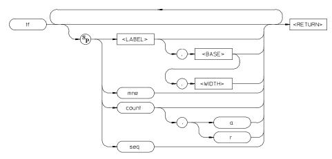
The **tf** command allows you to specify which pieces of information from the trace memory of the emulation-bus analyzer will be displayed by **tl** (trace list) commands.
