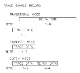
Trace Sample records are variant records which are components of the New Timing Data Record and More Timing Data Record. The structure of the Trace Sample Record depends on the count type field in the Timing Data Records.
