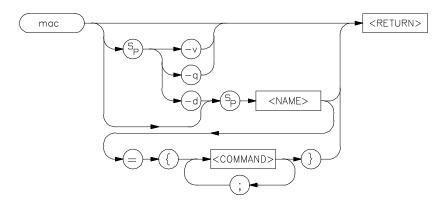
The **mac** command allows you to save a group of commands under a name of your choice. This allows you to instantly recall that command group by typing in the assigned name; the emulator will then preprocess the macro to expand the commands stored therein to a normal command line; the command line is then executed as usual.
