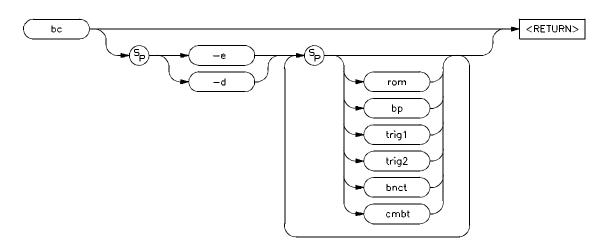
The **bc** command allows you to set break conditions for the emulation system. If no parameters are specified, the enable/disable status of all six break conditions is displayed.
