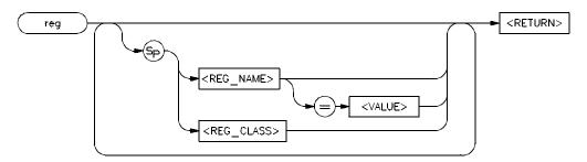
The **reg** command allows you to display and modify emulation processor register contents. Individual registers may be displayed or modified. Related groups of registers may be displayed. Combinations of display and modify are permitted on the same command line.
