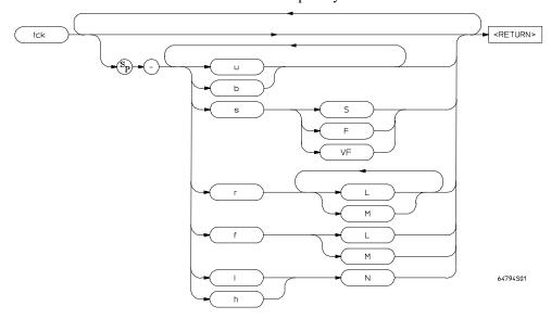
The **tck** command allows specification of clock qualifiers, master edges and maximum clock speed of the master clocks used for the emulation-bus analyzer. The clock speed selection has no effect in the deep analyzer.
