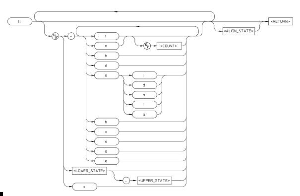
The  ${\bf tl}$  command allows you to display the current emulation-bus analyzer trace list information.
