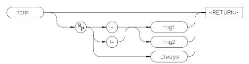
The **tarm** command allows you to specify an arming condition for the emulation-bus analyzer. You can specify the arm condition as the assertion of the trig1 or trig2 signals or as **tarm always**. The arm condition may then be used in specifying the analyzer trigger or in specifying branch conditions for the sequencer, as well as count or prestore qualifiers.
