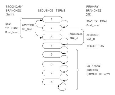
Here is how the analyzer can be set up to match this state diagram:
