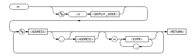
The **m** command allows you to display and modify emulation and target system memory. Options allow you to specify the display mode, specific address or addresses for display or modification, and the data values to be inserted.
