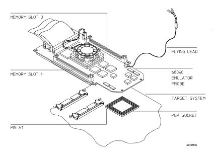
2 Insert the emulator probe into your target system socket. Make sure to align pin A1 of the emulator probe and your system socket.
