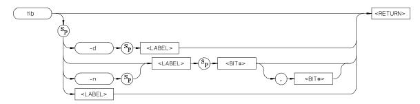
The **tlb** command allows you to define new labels for emulation-bus analyzer lines, as well as display or delete previously defined analyzer labels.
