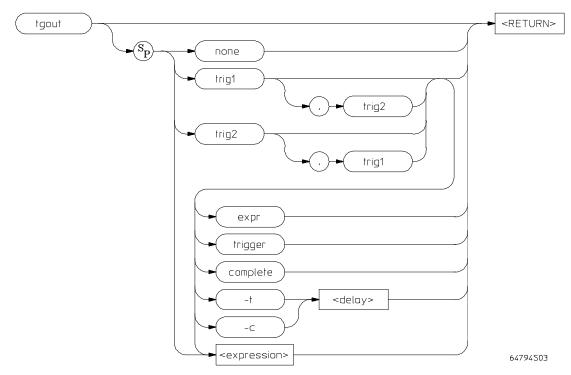
The syntax diagram above shows the syntax available when using the deep analyzer. If using the 1K analyzer, the **expr, trigger, complete, -t** and **-c** options are not available; by default, your trig1/trig2 choice selects the trigger function.
