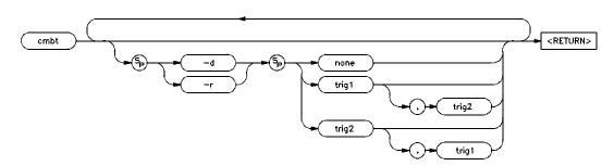
The **cmbt** command allows you to specify which of the internal **trig1/trig2** trigger signals will drive and/or receive the rear panel CMB (Coordinated Measurement Bus) trigger. You can specify the signals individually, as an ORed condition for drive, or as an ANDed condition for receive; or, you can specify that the signals are not to be driven and/or received.
