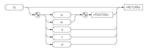
The **tp** command allows you to specify where the trigger state will be positioned within the trace list.
